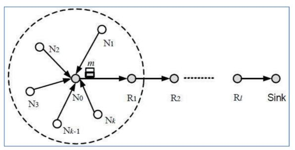
Fig. 1. Cooperative CNR-based authentication mechanism.
